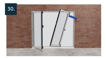
For track bound doors release the espag handle and slide the doors towards the hinged jamb until the central hinges are exposed. Remove the screws and remove the sash by supporting at the hinged jamb and sliding away from the hinged sash. This can then be removed by angling the sash until the top guide disengages from the track. Carefully lift the sash out of the bottom track until the roller is clear and place securely out of the way to prevent damage.
