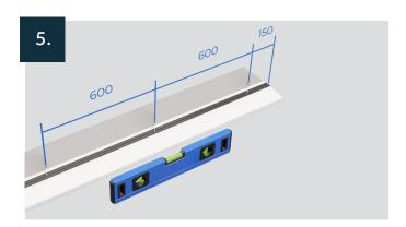
Fix 150mm from each end, and no more than 600mm between centres. Use a 1.8m level, laser level or suitable device to ensure the cill is level (+/-1mm per metre).
