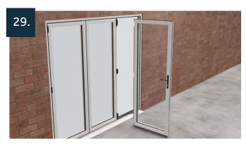
Starting with the single 'traffic' sash if available. Open and remove the screws from the hinges, fully supporting the sash while this is done. Lift carefully and place securely out of the way to prevent damage.
