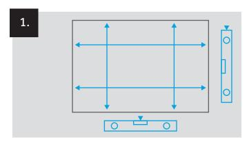
Ensure that all four sides of the aperture are plumb and square and identify any potential packing points.
