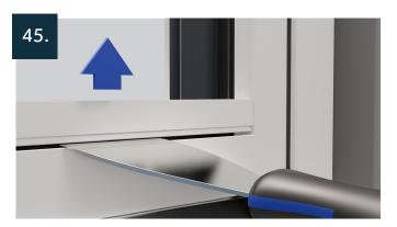
Push down on tool to disengage bead.
