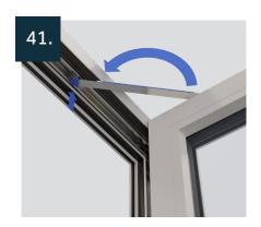
Open the sash to desired maximum opening angle, hold or wedge to keep it in place, and then position the restrictor arm to determine frame bracket location.
