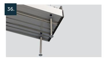
Secure the frame to the threshold using the supplied 4.8 x 55mm screws through the pre-drilled holes. Secure the top of the outerframe using the same method.
