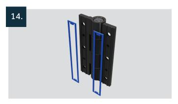
Hinge adjustment packers are available if required to square up the sashes in the frame, and each packer gives you 0.5mm of adjustment. Note: Maximum of 2 packers per hinge. Fit the necessary packers prior to fitting the hinge.
