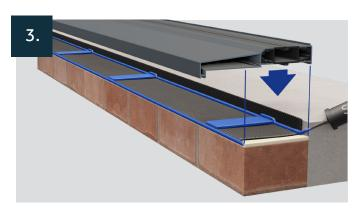
Add a damp-proof layer to prevent water ingress, running this 150mm up either side of the aperture. This needs integrating correctly with the structures original damp proof course. Ensure the cill is level and sufficiently packed to support the bi-fold along its full width. If the surface is uneven then a mortar bed may be necessary. If a mortar bed is not required then seal along edge using silicone sealant as shown.
