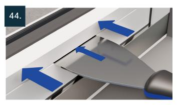
Push on upper edge of bead to tilt it backwards to allow you to slide a tool between the bead and sash profile.
