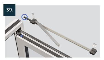
Locate datum bar against sash insert and screw the door restrictor into position on the sash using four 4.3 x 25mm countersunk screws.
