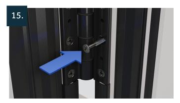
Fit final fixing screws in hinges once all adjustments have been made.
