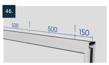
Fix frame extender 150mm from ends and max 500mm between centres using  $4.3 \times 55$ mm countersunk screws (or  $4.3 \times 35$ mm countersunk screws if the extender is flipped with the thermal break against the frame)
