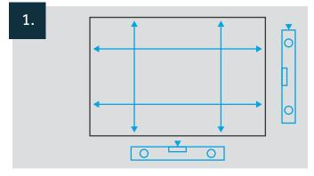
Ensure that all four sides of the aperture are plumb and square and identify any potential packing points.
