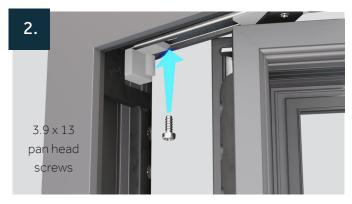
Once the sash is firmly located it will be held firmly in place allowing you to fix the hinge using  $3.9 \times 13$  pan head screws. Once complete test for correct operation and repeat as required.
