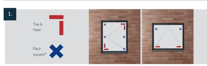
Fit the glazed unit into the sash and pack / toe & heel in the appropriate places using glazing packers as shown. Toe & heeling should distribute the weight of the glass correctly to ensure the window is square and aligned. Using glass packers at the opposite corners of the sash as shown, creates diagonal support across the glass unit, ensuring the window operates correctly.
