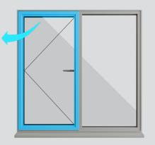
**IMPORTANT:** If large windows have arrived to site with the sashes installed you may want to remove them before installation to stay within safe manual handling limits.
