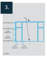
Additional fixings required for frames over 1.8m top and bottom as shown, in line with industry codes of practice.
