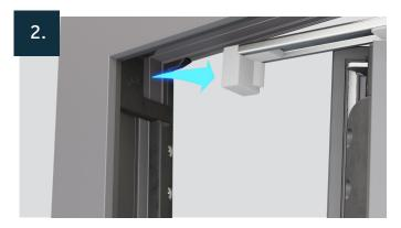
Holding the sash securely, tilt the hinges away from the corner hinge locators and lift out.
