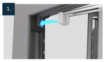
Place the back edge of the hinges in the corner hinge locators, and then rotate the sash forward locating the front edge of the hinge into the run up ramps.
