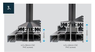
Fix through the cill into the window frame using countersunk PVCu screws as shown above, taking care that they do not break into the internal glazing rebate.
