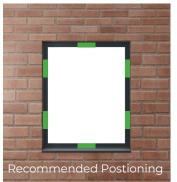
The SH128 external/internal Glazing clip base should already be fitted as shown above.
