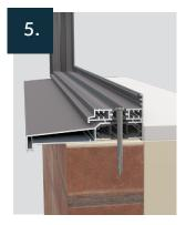
Fix the frame into the aperture using suitable 100mm frame fixings to suit construction material.
