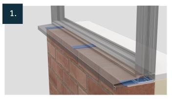
Pack under cill and window jambs and seal along the aperture cill in preparation for installation. It is good working practice to set outer frame 30mm in from the front face of the brickwork.
