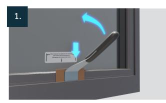
If already fitted, release the sash by locating the dummy sash packer using the release tool. Press down firmly onto the paddle plate before rolling forward onto the sash to disengage the lock, ensuring you have put protective padding in place to protect the sash.
