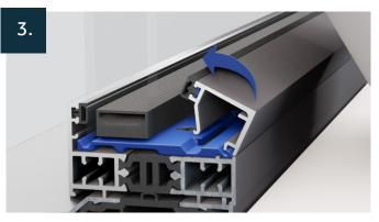
Fit the top bead first to prevent the glazed unit from falling out of the window, continue to fit the bottom bead and then the sides being careful not to scratch the powder coated finish.
