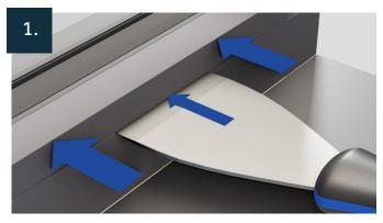
Press the top edge of the bead toward the glass, creating a gap between the bead and the frame/ sash.
