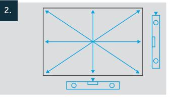
Check that the cill is level and provides a solid base to ensure it will not cause distortion of the window. Note: The window should be packed under the cill and frame jambs to provide sufficient support.
