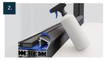
Spray the glass unit with a mild soap/water mix or glass cleaner to prevent the gasket sticking while the bead is being fitted.
