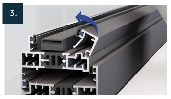
Start by locating the front leg of the bead into the receiving channel and rotate the bead until it 'clips' into place. Fit the top bead first to secure the unit. Continue to fit the bottom bead and then the sides being careful not to scratch the powder coated finish.
