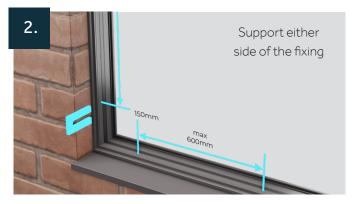
Pack around the frame using full-width packers ensuring that it's square and level and ensuring a 5mm gap is maintained. Drill pilot holes around the frame at min 150mm from corners and min 600mm centres in between, ensuring at least 2 fixings per side.
