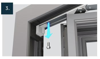
Make sure you have a safe and protected surface to lay the dummy sash once you've removed it. Start by unscrewing the sash.
