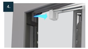
Holding the sash securely, tilt the hinges away from the corner hinge locators and lift out.
