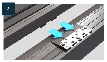
Once located give a firm push on the sash to engage the teeth and lock the sash into the frame. Make sure to push firmly on both devices to ensure good gasket compression. Check that the gap between the sash and the outer frame is consistent from left to right and that everything is parallel.
