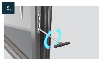
If you need to adjust the compression on window sashes, to ensure they open with minimal effort but maintain a tight seal when closed. Adjust the locking pins on the espag lock using a 4mm allen key.
