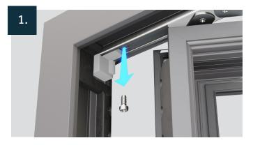
Remove the screws holding the hinge to the frame while holding the sash securely.
