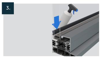
Spray the glass unit with a mild soap/water mix or glass cleaner to prevent the wedge gasket sticking to the frame or glass.
