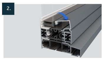
Rotate the back leg of the bead into the frame then clip the front leg into position.
