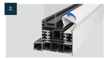
Start by locating the front leg of the bead into the receiving channel and rotate the bead until it 'clips' into place.
