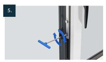
If you need to adjust the compression on window sashes, to ensure they open with minimal effort but maintain a tight seal when closed. Adjust the locking pins on the espag lock using a 4mm allen key.
