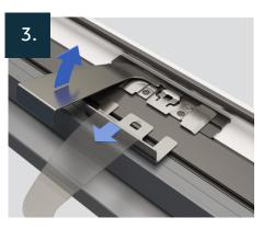
Place the handle part of a second de-glazing tool between the clip and the glass and pull the clip out as shown.
