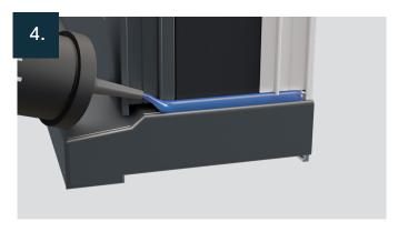
Seal with silicone along the edge where the cill meets the frame.
