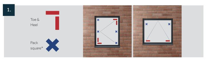
Fit the glazed unit into the sash, and pack / toe & heel in the appropriate places using glazing packers as shown.
