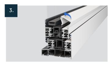
Start by locating the front leg of the bead into the receiving channel and rotate the bead until it 'clips' into place.
