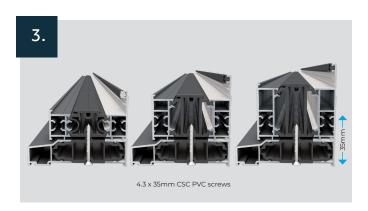
Fix through the cill into the window frame using countersunk PVCu screws as shown above, taking care that they do not break into the internal glazing rebate.
