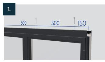
Fix frame extender 150mm from ends and max 500mm between centres using  $4.3 \times 55$ mm countersunk screws (or  $4.3 \times 35$ mm countersunk screws if the extender is flipped with the thermal break against the frame)
