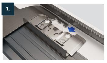
Place the de-glazing tool under the sealed unit to the back of the window section as shown. Then slide the de-glazing tool to the left / right until it meets the Securi-clip and pull towards you.
