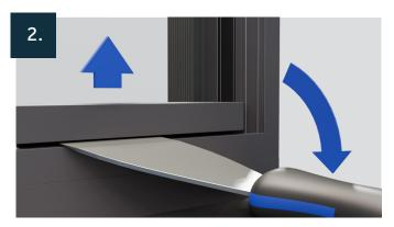
Using a thin pallet knife or appropriate tool, insert the tool in the gap created and leaver away from the bead to disengage from the fixed profile.
