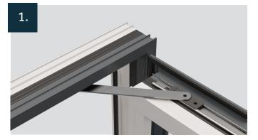
Locate datum bar against sash insert and screw the door restrictor into position on the sash using four 3.9mm x 16mm pan head self drilling screws.
