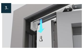
Make sure you have a safe and protected surface to lay the dummy sash once you've removed it. Start by unscrewing the sash.
