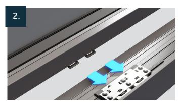
Check that the gap between the sash and the outer frame is consistent from left to right and that everything is parallel. Now push firmly closed.
