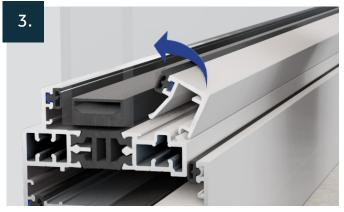
Start by locating the front leg of the bead into the receiving channel and rotate the bead until it 'clips' into place. Fit the top bead first to secure the unit. Continue by fitting the bottom bead and then the sides, being careful not to scratch the powder coated finish.
