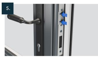
If you need to adjust the compression on door sashes, to ensure they open with minimal effort, but maintain a tight seal when closed. You can increase the contact pressure between the sash and frame as required by using the two machine screws indicated.
