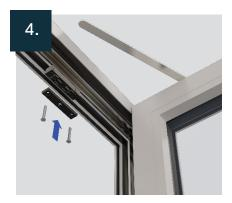
Mark & drill two 2.5mm pilot holes through the head track & fit the frame bracket and track location packer with two 3.9 x 30mm countersunk screws.
